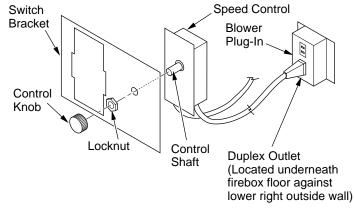
Figure 26 - Attaching Speed Control to Firebox
